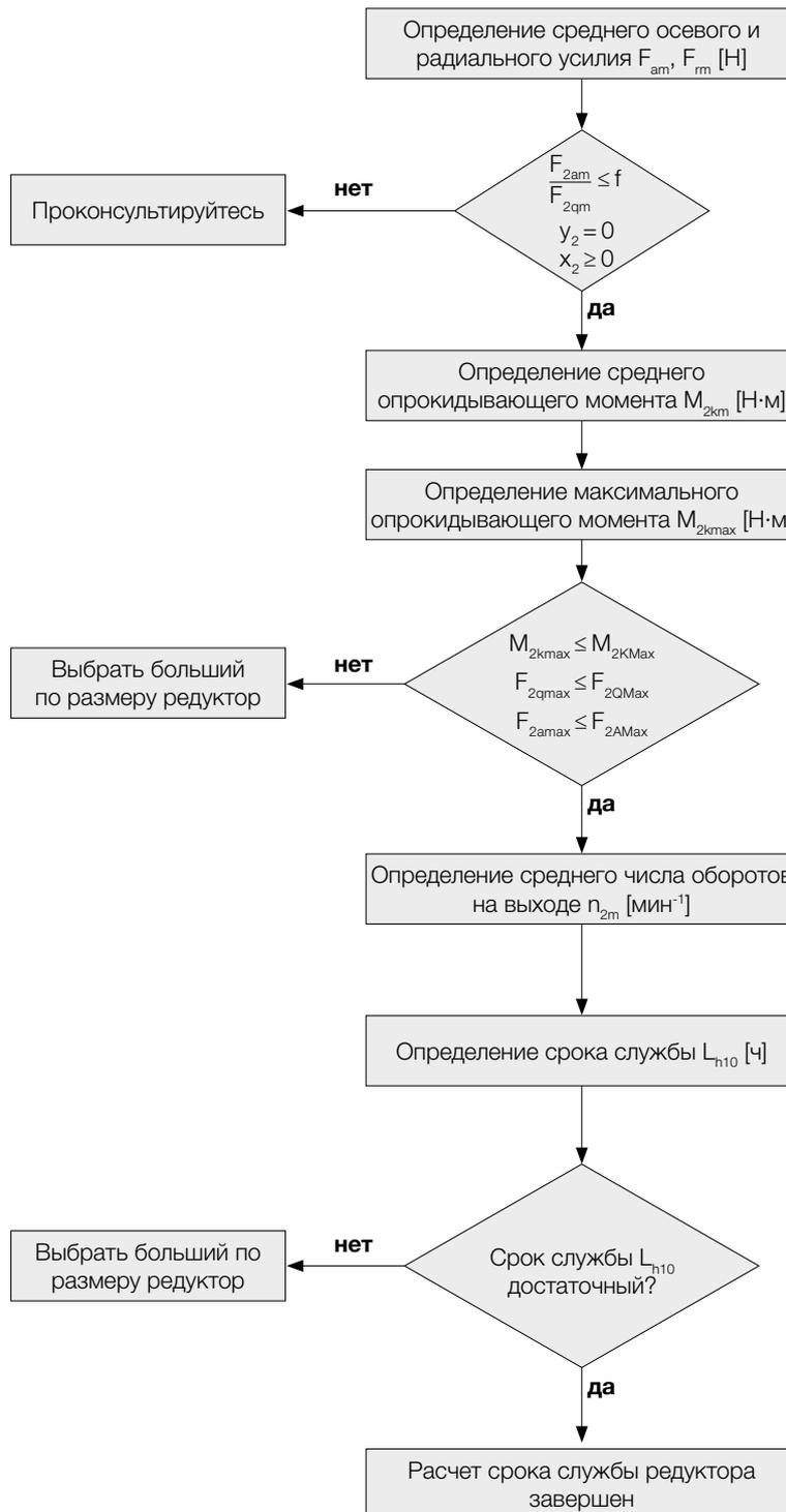
$$F_{2am} = \sqrt[3]{\frac{|n_{2b}| \cdot t_b \cdot |F_{2ab}|^3 + \dots + |n_{2n}| \cdot t_n \cdot |F_{2an}|^3}{|n_{2b}| \cdot t_b + \dots + |n_{2n}| \cdot t_n}}$$
