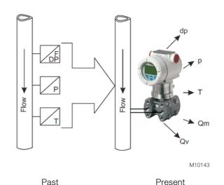
Fig. 1: Flow measurement - past and present
