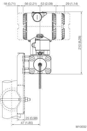
Fig. 8: Flat bracket for pipe mounting - Barrel housing
