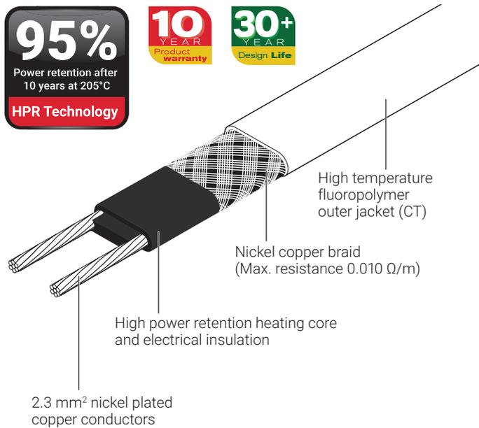
The nVent RAYCHEM HTV self-regulating heating cable is designed for freeze protection or process temperature maintenance of pipes and vessels with very high continuous operating temperatures (205°C).
