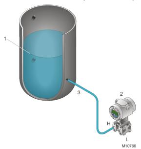
Fig. 23: Liquid level measurement on open tanks
