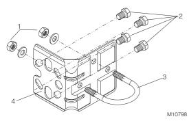
Fig. 14: Detail view of the mounting bracket, B2, for pipe and wall installation.
