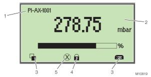
Fig. 31: Process display (example)
