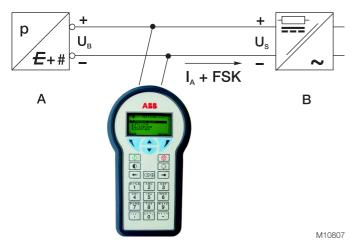
Fig. 36: Communication structure with handheld terminal A Transmitter | B Energy supply (communication resistor integrated in the feed device)
