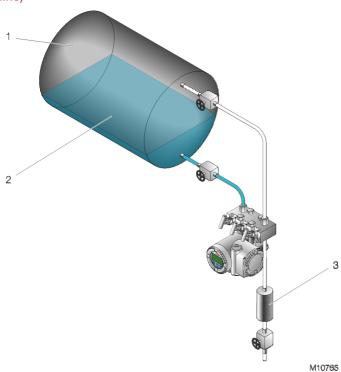
Fig. 21: Fill level measurement on closed tanks (gas-filled impulse line)
