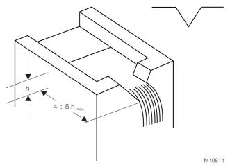
Fig. 43 V measuring weir
