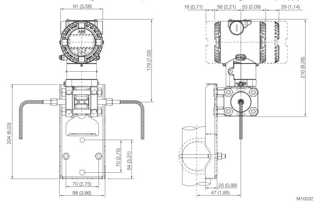
Fig. 8: Flat bracket for pipe mounting - barrel housing
