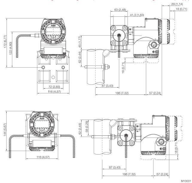
Fig. 7: Pipe mounting - DIN housing
