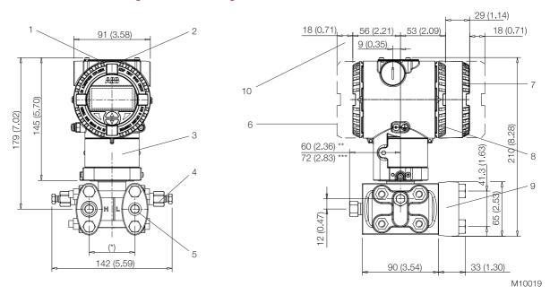
Fig. 9: Barrel housing - horizontal flanges
