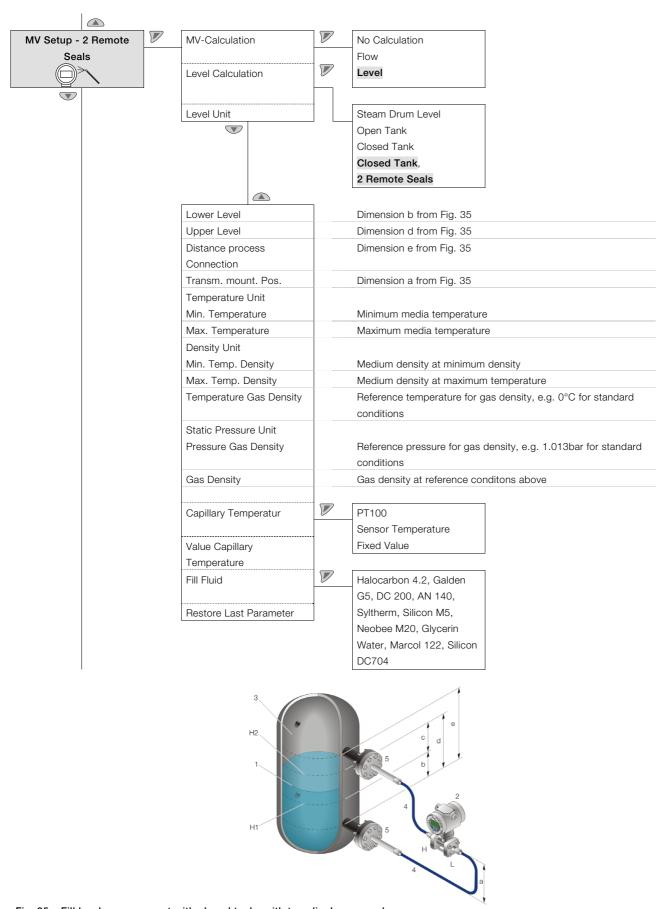
Fig. 35: Fill level measurement with closed tanks with two diaphragm seals
