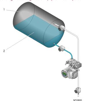
Fig. 22: Level measurement on closed tanks (liquid filled impulse line)
