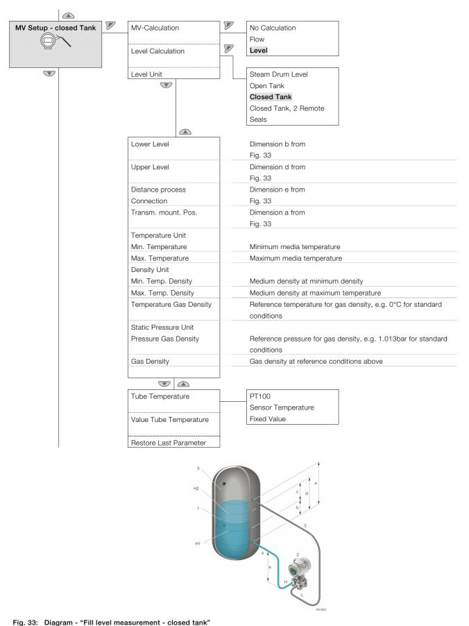
H1 The lower level to be measured | H2 The higher level to be measured
