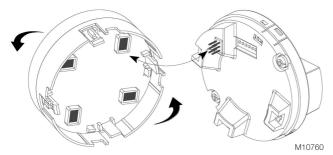
Fig. 17: Rotating the LCD display
