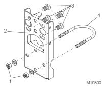
Fig. 15: Detail view of the mounting bracket, B5
