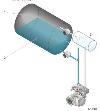
Fig. 24: Fill level measurement on the steam boiler
