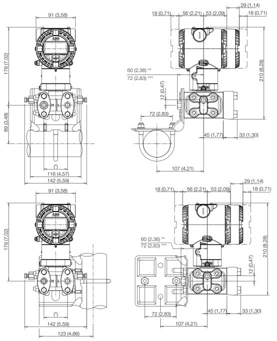
Fig. 11: Pipe mounting - barrel housing
