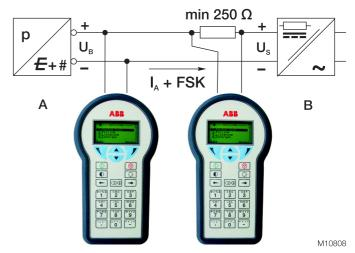
Fig. 37: Connection example with communication resistor in the connecting line
