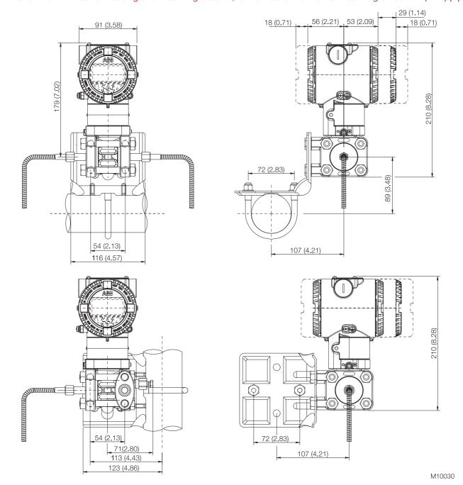
Fig. 6: Pipe mounting - barrel housing
