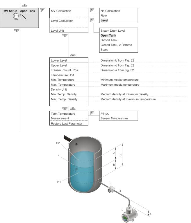
Fig. 32: Diagram - "Fill level measurement - open tank"
