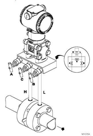
Fig. 20: Flow measurement of gases or liquids A High-pressure valve | B Low pressure valve | C Equalizing valve | H High pressure side | L Low pressure side
