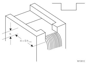
Fig. 41: Rectangular measuring weir
