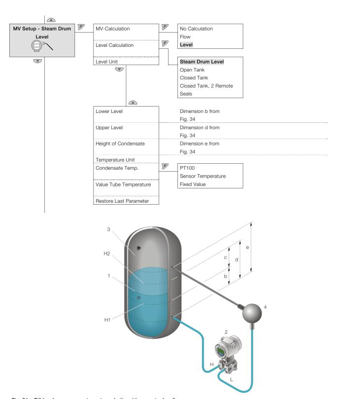
Fig. 34: Fill level measurement on steam boilers (drum water level)
