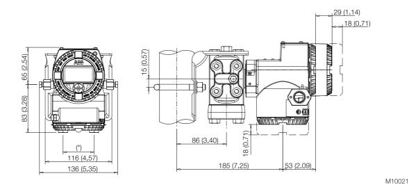
Fig. 12: Pipe mounting - DIN housing
