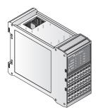
In addition to hardwiring an RTD directly into a Heat Trace Control module, RTDs can be wired to Input/output modules (NGC-40-IO) within the panel and assigned to heat-tracing circuits through software. This means that a NGC-40 system can be optimised for the specific application needs. Each IO module accepts up to four additional RTD inputs.
