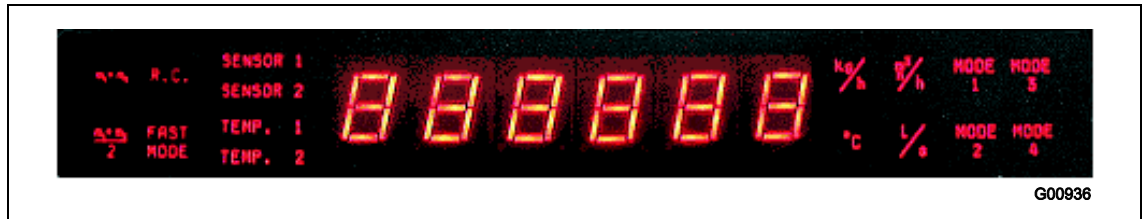
Fig. 15: Display of the supply / evaluation unit (lamp test during switch-on)
